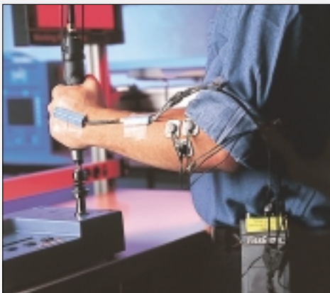
A Q2 screwdriver in test for measurement of torque reaction, muscle efforts, temperature conductivity of tool handle and total work performance.
